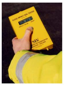
The CIST/882 Readout Unit is held in the hand during testing. It displays readings of Impact Value (IV) and also shows the number of times that the hammer has been dropped during each test operation. Unlike previous models the user does not need to keep the 'On' button pressed during testing.
