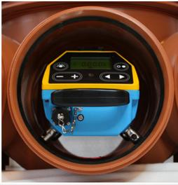
**Flat bottem for easy flow.** Combined with a weight of 4.5KG gives staying power even when working small diameter live pipes. **4.5KG = Stability.**
