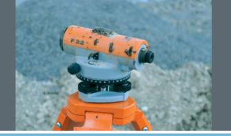
The F-levels feature first-class optics with 24x, 28x or 32x magnification, a top-quality magnetic-damped compensator and a modern design. Just right for use under tough conditions.
